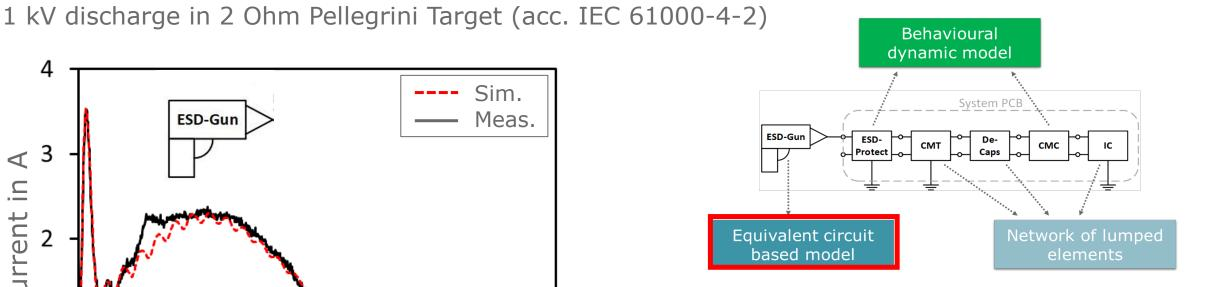
Entire shape of ESD generator model is replicated with very high precision and corresponds to IEC61000-4-2
