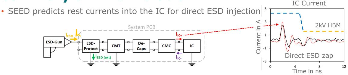
• System Model can be also extended for transient analysis of coupled ESD injections
