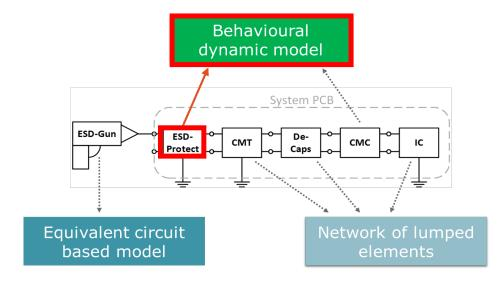
The ESD Protection is modeled using TLP. Not only the static behavior is modeled but also the dynamic behavior using peak voltages of each TLP pulse
