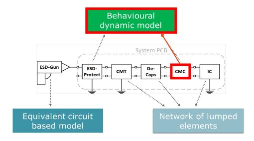
The CMC Protection is modeled using TLP measurement similar to the modeling of the ESD device.
