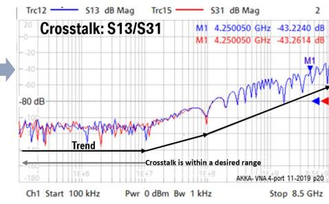
Almost no crosstalk effects below 10MHz; Increase of 10dB/decade from 10 to 100MHz Increase of 15 to 20dB/decade above 100MHz → no issue for classic bus system
