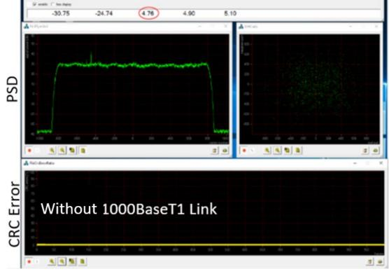
➔ DAB is prone to interferences from the 1000BASE-T1 data traffic
