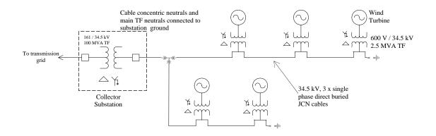
Figure 1: Typical Wind farm network- single line diagram (only a few turbines are shown)
