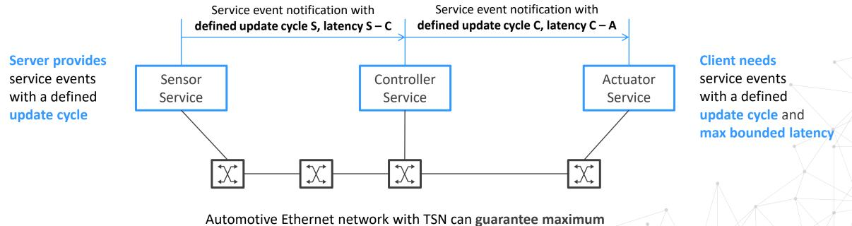
Automotive Ethernet network with TSN can guarantee maximum bounded latencies for control data streams by separating the streams into up to 8 traffic classes and applying traffic shaping
